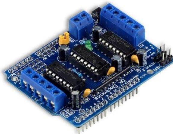
This is a commonly used DC motor drive module, using L293D chip with small current DC motor driver. The pins are made compatible with Arduino which is easy to use.
